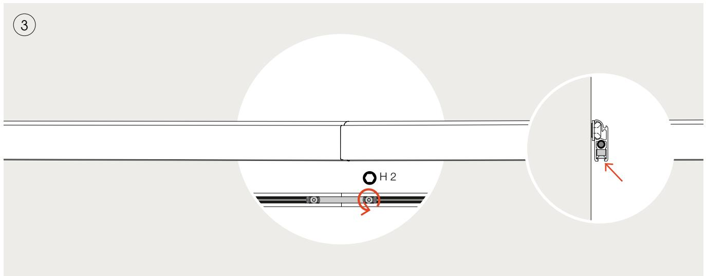
Press the sections of track together. Screw the other side of the track into place.
