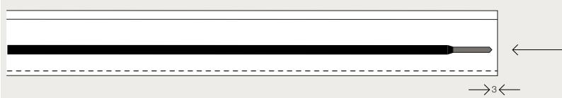
Re-insert the inner conductor into the track profile so that the end of the inner conductor is offset 3 mm on the inside on both sides of the track.
