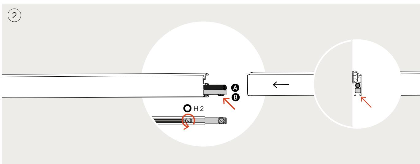
Slide the electrical connector (**A**) onto the inner conductor (**I**) of the first section of track. Insert the mechanical connector (**B**) into the track, as indicated, and screw firmly into place.
