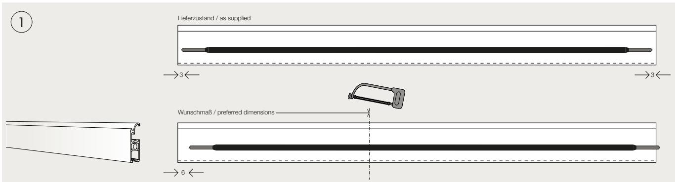
Position the inner conductor on the side not to be sawn so that it ends 6 mm short of the end of the track profile. Saw the track and the inner conductor together. Use a mitre saw to ensure a straight cut.
