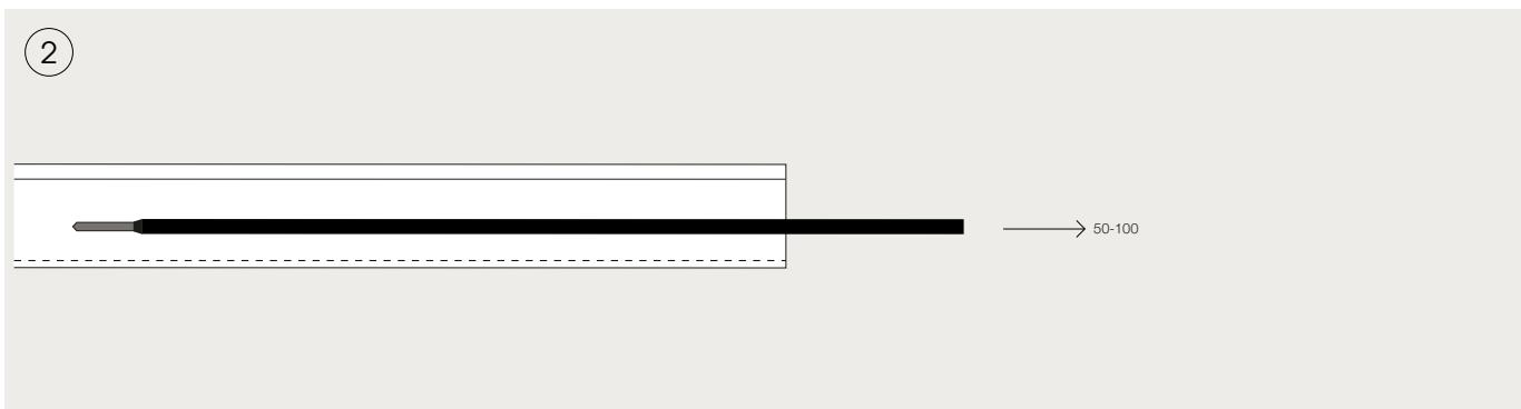
Push the inner conductor with the protective insulation approx. 50 to 100 mm out of the profile.
