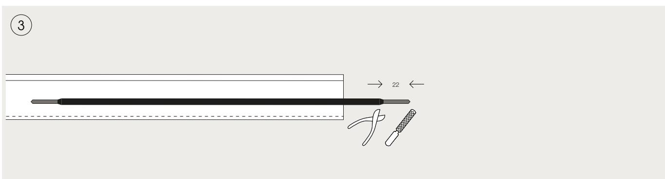
Strip 22 mm, trim carefully (taper) so as not to damage the contact interfaces in the electrical connectors.
